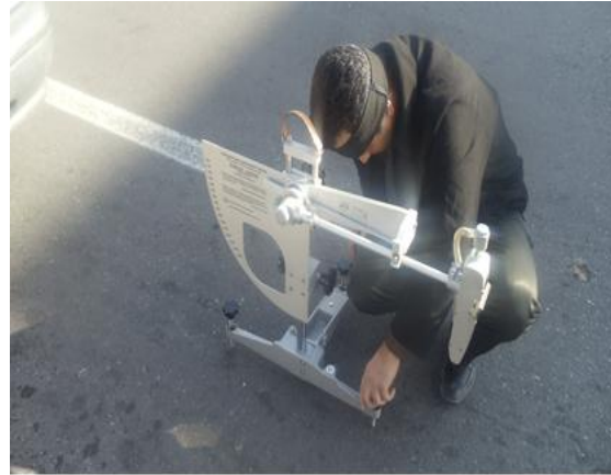
Figure 3. British pendulum test on conventional asphalt in Tehran.
